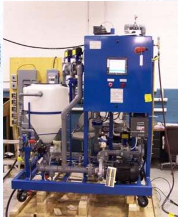
Field Evaluation ASCF 2 nd stage concentration & lower volume processing 1000 liters/shift
