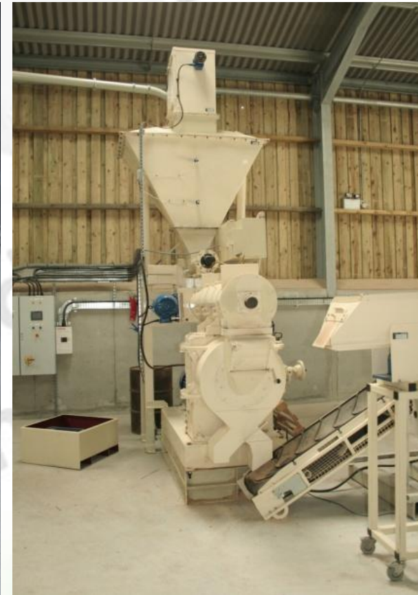
Dry processing: Pellet mill
